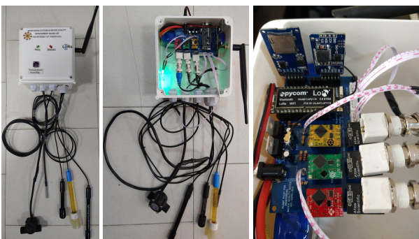
Figure 10. Physical detail of the IoTMonitor-WQ platform installed at the water quality parameter recording points.
