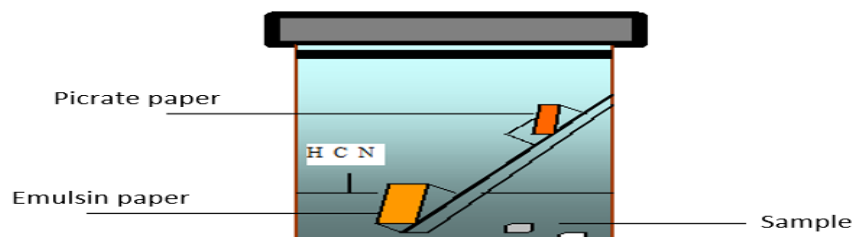
Figure 2. Device for measuring with picrate paper. Source: Arrazola et al. (2015)
