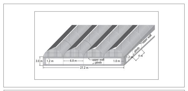
Figure 2. Section of the isometric drawing of greenhouse 3 and dimensions of the front and lateral ventilation areas
