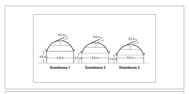
Figure 1. Dimensions of the gates of the top rear of the three greenhouses.
