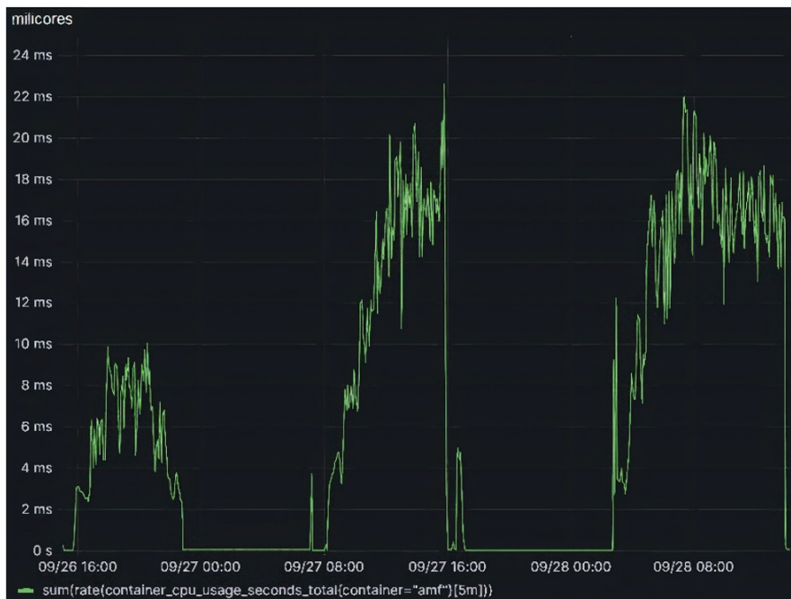
Figure 7. Total CPU usage for reactive, predictive, and self-scaling policies scenarios, respectively, using My5G-RanTester.
