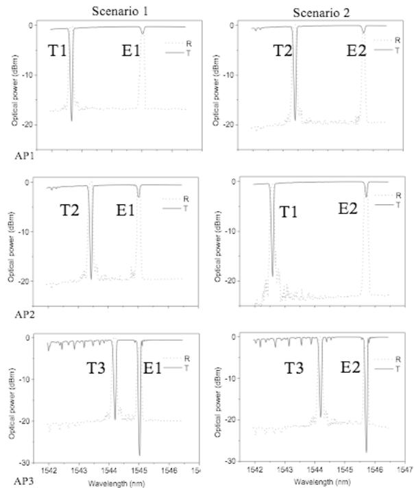
**Figure 5.** Experimental results. FBG responses for three access points featuring tunable and equalized FBGs in two scenarios
