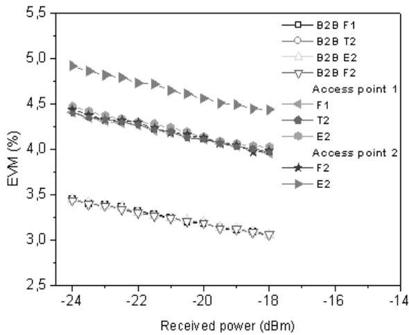
**Figure 3.** Signal degradation for the channels dropped by AP1 and AP2 featuring RF services
