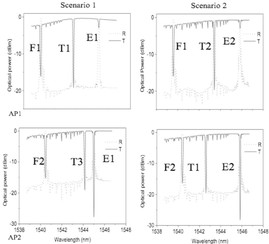
**Figure 2.** Experimental results. FBG responses for two access points featuring fixed, tunable and equalized FBGs in two different scenarios
