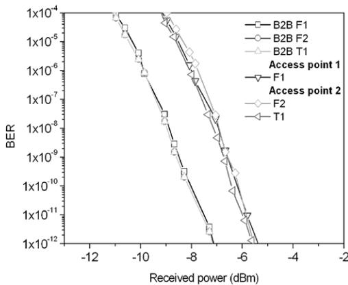
**Figure 4.** Signal degradation for the channels dropped by AP1 and AP2 featuring baseband services
