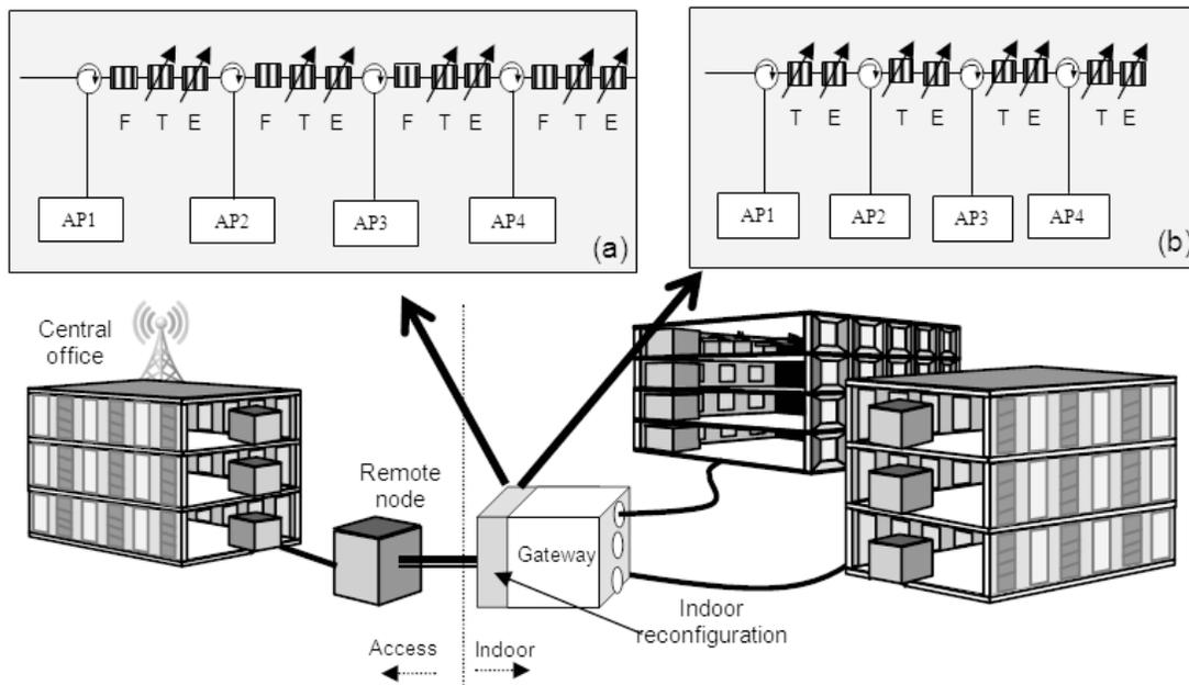
**Figure 1.** Reconfigurable architectures for indoor scenarios. (a) Featuring fixed (F), tunable (T) and equalized (E) FBG. (b) Featuring tunable (T) and equalized (E) FBG
