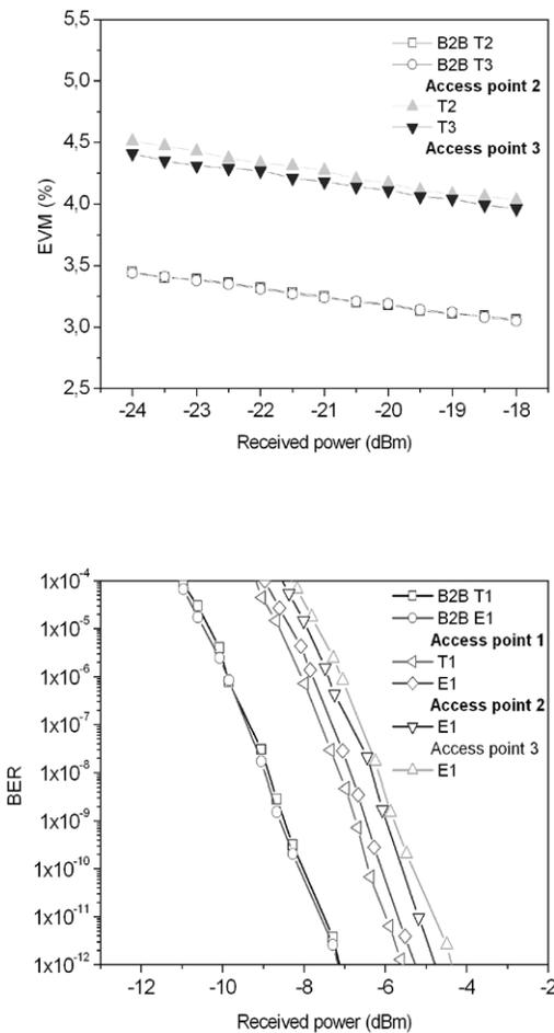
**Figure 6.** Signal degradation for the channels dropped by AP1, AP2 and AP3 featuring RF and baseband services
